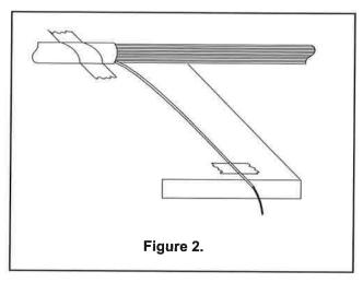
6.4 Wipe all gel from the exposed fibers using a gel cleaner.
